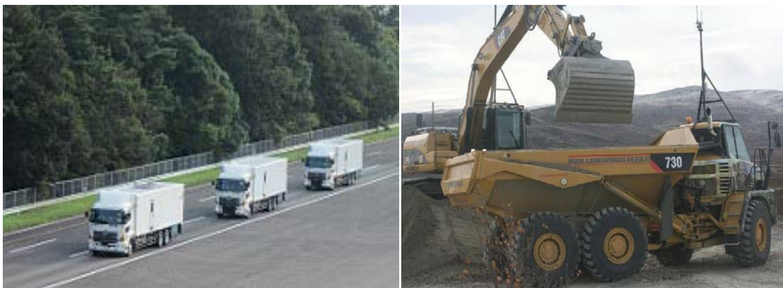
Figure 1.4 Left: Three trucks with one lead driver conducting a test in 80 km/h (photo: NEDO). Right: Remotely controlled shovel and dumper at Hjerkins firing range (photo: Geir Olav Slåen).
