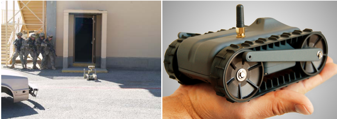
Figure 1.2 Left: Support UGV (Packbot) assisting soldiers in operations. Right: LANdroids (photos: iRobot Corporation).
