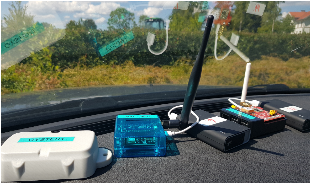
(a) LoRaWAN devices deployed for Drive 1 (one of two vehicles shown).
