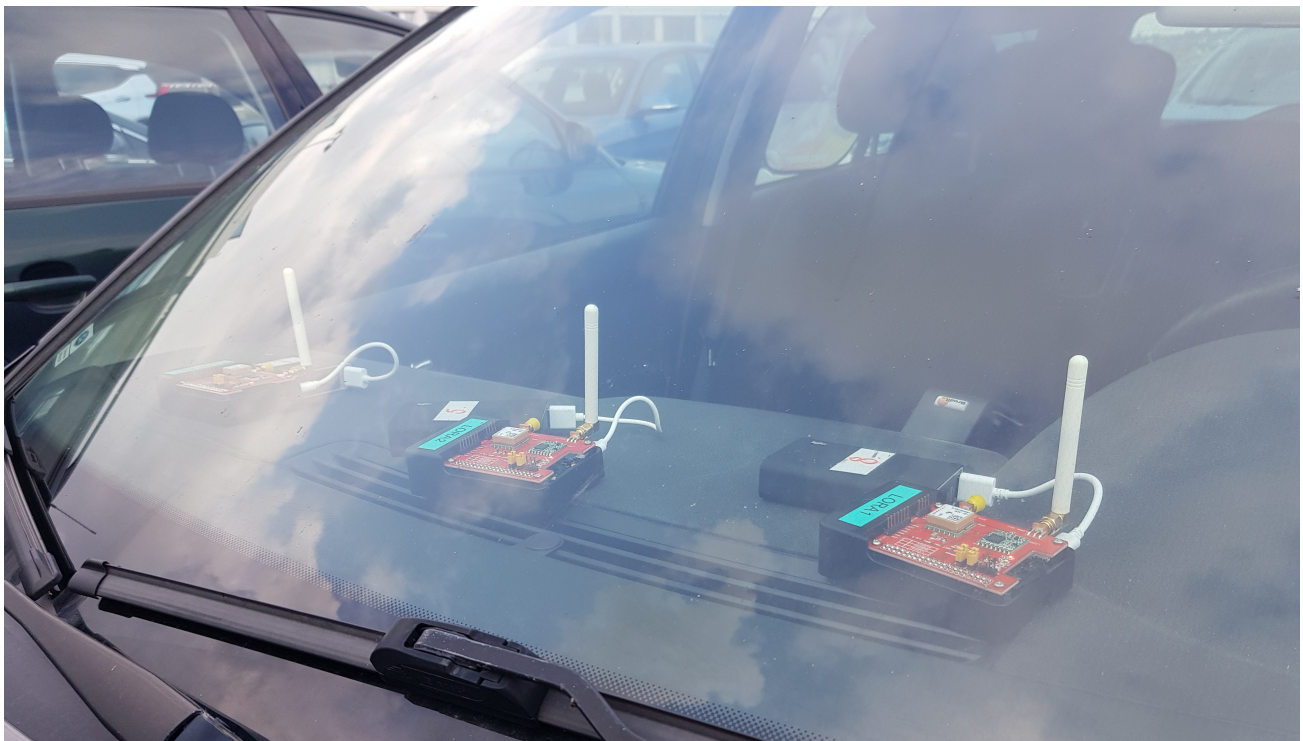
(b) All three Raspberry Pi 3 with Dragino HATs deployed in one vehicle for Drive 3.
