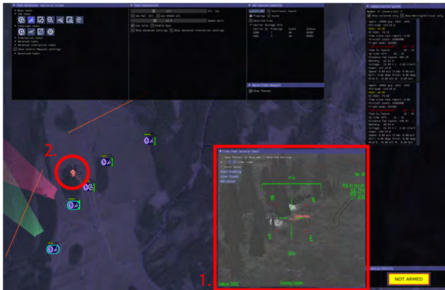
Figure 6.1 Valkyrie GCS with a synthetic sensor image (1) detecting a group of synthetic vehicles in a forest (2). This observation is pushed to NORCCIS on TYR.
