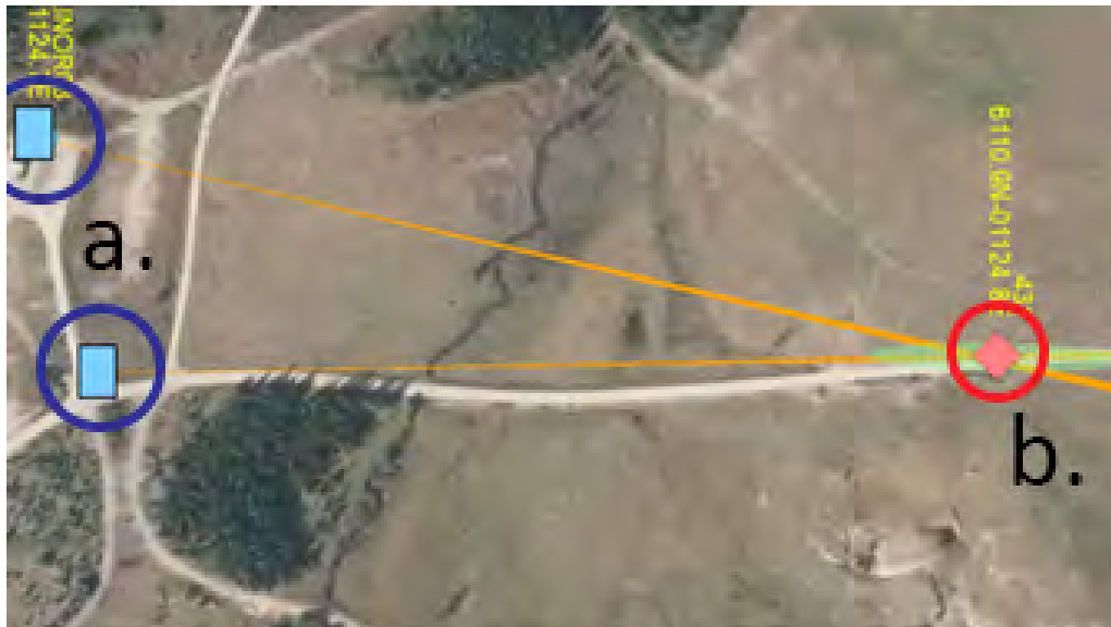
Figure 7.2 A tactical map image from LandX23 showing two Elinor sensors (marked a.) with a geolocalized radar (marked b.) at the intersection of the two bearing lines.
