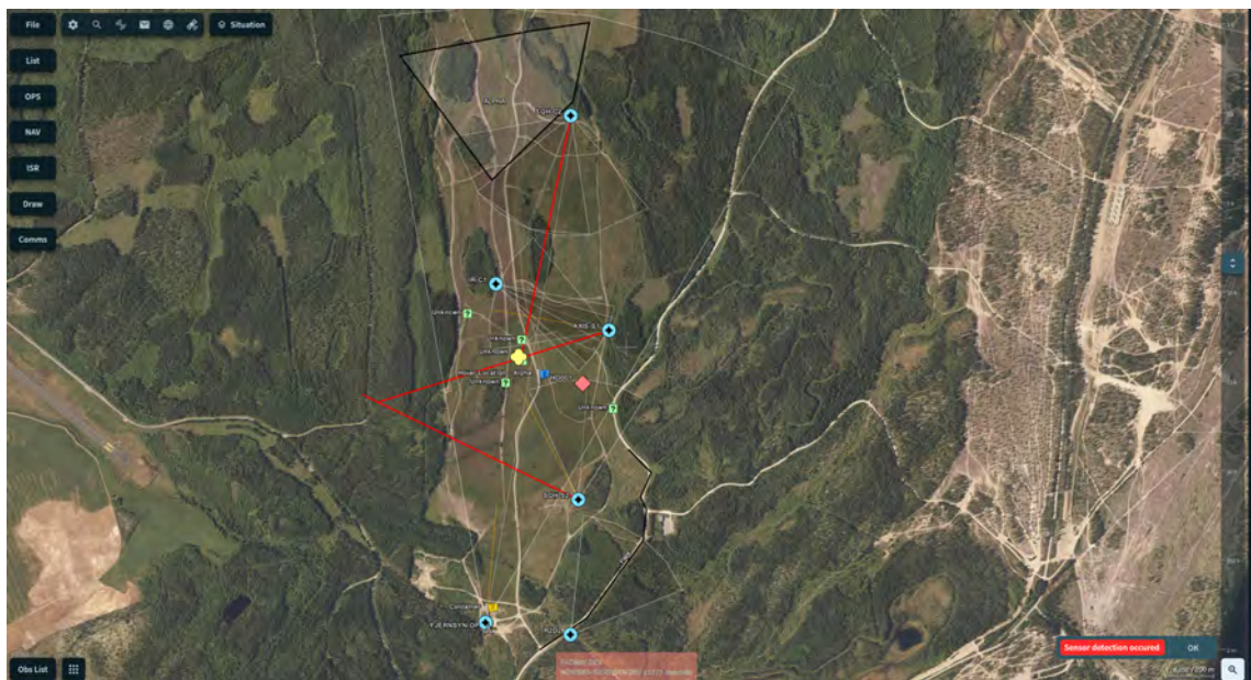
Figure 4.4 Screenshot from NorBMS showing sensor nodes (as blue circles) sensor directions (as sectors from sensor nodes), detections (as red lines emitting from sensor node), radar tracks (as green squares), detections (as yellow “flower”) and a target (as red diamond)
