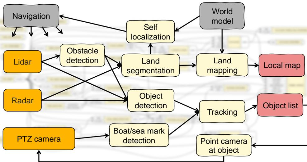
Figure 1.2 Outline of main features in the processing pipeline of Warpath ASV. Note that navigation is integral to all processes, hence the simplified representation.
