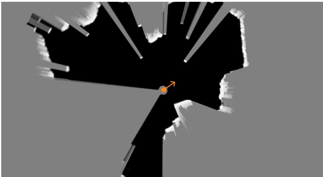
Figure 3.2 Log odds plot of “not water” vs “water” from the radar mapping stage. Our vessel has position and heading as given by the orange dot with arrow. Black indicates “water”, white indicates “not water”, and 50% gray indicates that we have no information. As can be seen from the gray “shadows” we have no confidence in radar returns that are obstructed by nearer returns. The gray triangle behind our vessel is due to the  $\sim 64^\circ$  rearward blind-zone.
