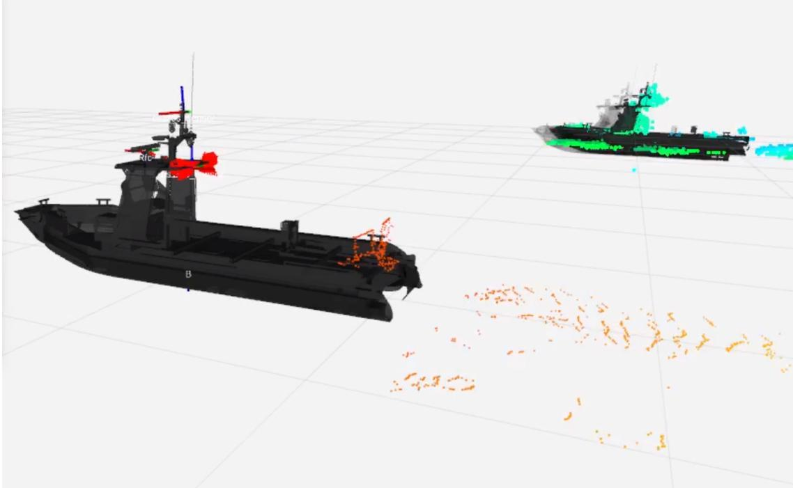
*Figure 2.2 Visualization of the Ouster OS-2 lidar pointcloud. The data is captured from the vessel on the left, which observes the cooperating vessel on the right. Lidar returns are shown as the dots color-coded by distance.*
