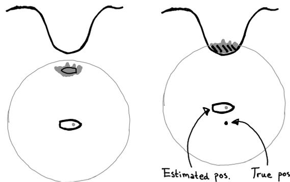
Figure 5.4 Localization bias when land is out of range of the radar. The method may incorrectly recognize the detection of the oncoming vessel as coastline and thus match the detection with the headland above. The low amount of radar returns will yield low confidence.
