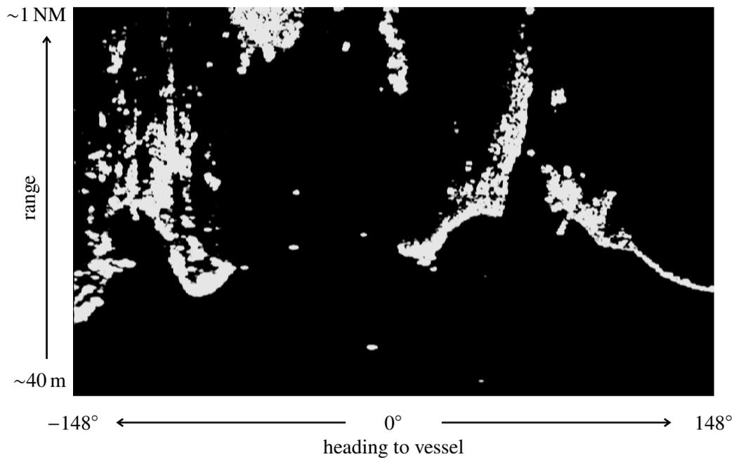
*Figure 2.1 Raw polar plot from the HALO-3 Radar. White areas represent strong radar responses, while black represents no response. The large continuous shapes are generally caused by land formations. Smaller free-standing blobs can indicate smaller objects in the water, but many of the small blobs seen here are just clutter.*
