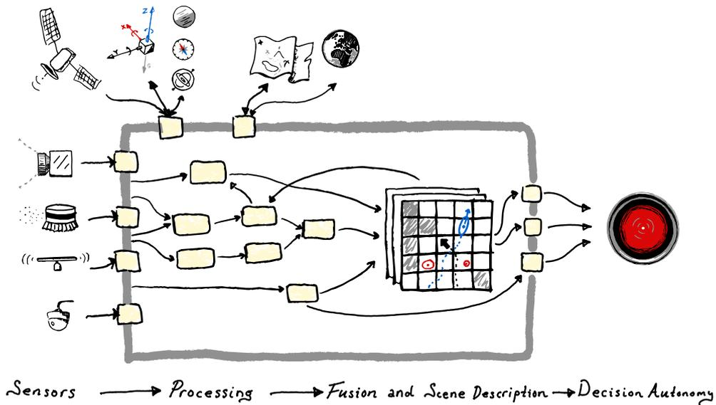
Figure 1.1 Architectural overview of Warpath. Warpath interfaces several sensors, navigation components, and prior map sources, whose data is fused in a processing graph. The resulting output is self-localization, a land/sea map, and a list of tracked objects, which is handed over to the decision autonomy (HAL).
