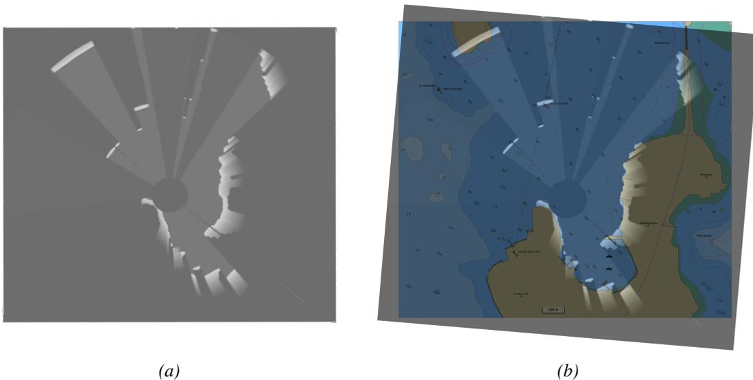
Figure 5.1 Absolute geographical localization by coastline matching. Fig. (a): The result from coastline detection in a single radar sweep. Fig. (b): The same plot overlaid a georeferenced sea chart. Even though we have noise and detections of sea markers in the water, the method is able to align the two images.
