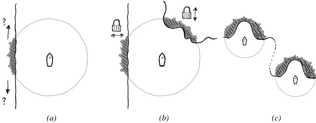
Figure 5.3 Land features that may influence the result. Fig. (a): With land formations like this, there will be a potentially large uncertainty in position along the direction of travel, as any position would yield a good match. Fig. (b): Detections in multiple directions and land formations with more unique features will give better results. Fig. (c): Similar looking land formations can give a good match locally, but result in an incorrect position globally.
