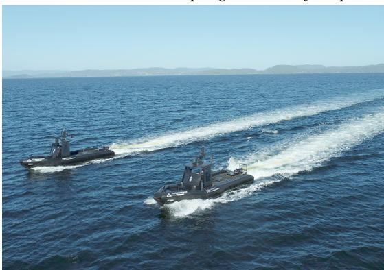
(e) September 2021: Odin and Frigg in tight formation based on fused lidar tracking and telemetry while towing a closed loop influence sweep [12].
