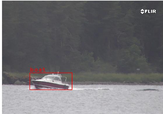
(b) June 2018: Initial tests with convolutional neural networks (CNN)-based boat detection in images from the FLIR M400 PTZ camera. Even stock models achieved surprisingly good results.
