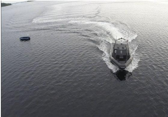
(a) Aug. 2017: An uncrewed Odin, seconds after autonomously performing an evasive manoeuvre against a fused radar+lidar track during a demonstration near Kongsberg Maritime, Horten.
