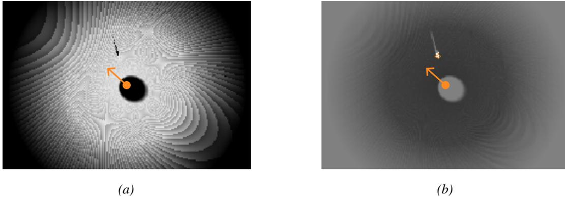
Figure 3.1 Feature images used in the lidar detection and mapping pipelines. Our own vessel has position and heading as given by the orange dot with arrow.
