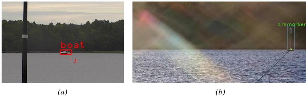
Figure 7.1 Detection of a boat (a) and a sea marker (b) in daylight images. The detector in (a) [15] was trained on the stock MS COCO dataset [19], while the detector in (b) [16] was also trained on a private dataset focusing on Norwegian sea markers [20], [21]. Both figures are from work carried out in 2017 – 2018.
