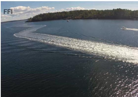
(c) June 2018: Odin's wake from autonomously performing a COLREGS-compliant manoeuvre after detecting a head-on-head situation with the small boat "Småen" in the top-right corner of the photo.
