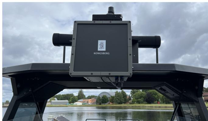
Figure 7.2 Phased array radar from Kongsberg Seatex mounted on Frigg.
