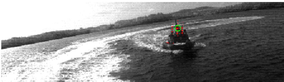
Figure 4.3 Ambient near-IR image from the Ouster OS2 lidar observing the cooperating vessel. Specular reflections are marked in red, while diffuse and ambient light are rendered as grayscale. The actual retroreflector lies underneath the strongest return (inside the green circle), while the weaker red dots result from blooming around the reflector. We use the strongest return as the detection.
