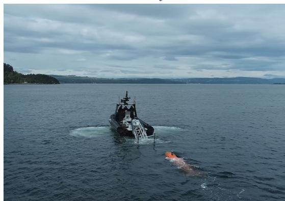
(f) May 2022: Frigg autonomously moving into position for recovery of Hugin AUV, based on fused lidar tracking and telemetry [13].
